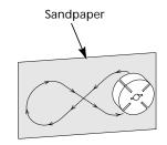
Figure 20 - Sanding Rotor
